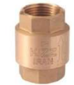
شیر یکطرفه فتری Spring Check Valve Model: KIZZIRAN 507 Material: Brass Size: 1/2~3 inch W.P. : 1/2~1 inch 16 bar 1 1/4~2 inch 12 bar 2 1/2~3 inch 8 bar
