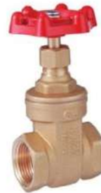
شیر کشویی Gate Valve Model: KIZZIRAN 500 Material: Brass Size: 1/2~3 inch W.P. : 1/2~2 inch 16 bar 2 1/2~3 inch 20 bar
